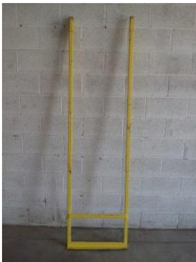
4. Main lower support bracket with flanged anchor attached
